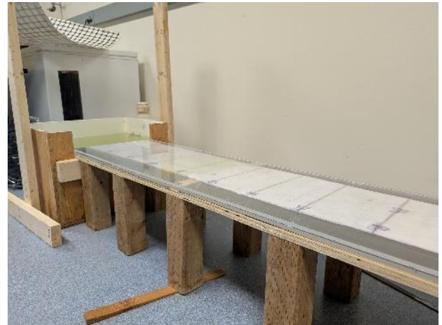
Figure 4. Table for modified horizontal wet front movement test
