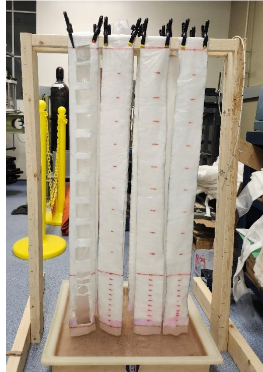
Figure 2. Capillary rise test equipment
