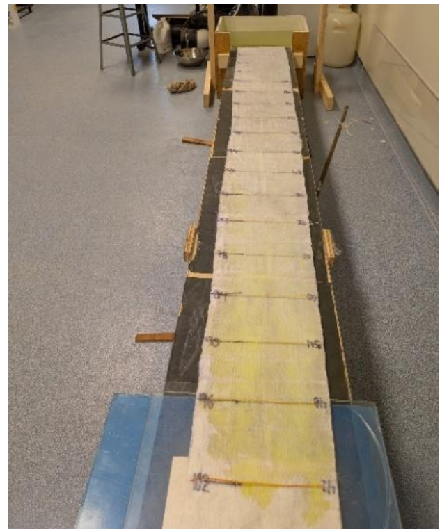
Figure 5. Horizontal wet front movement test without load
