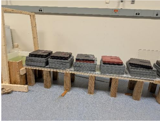
Figure 6. Horizontal wet front movement test with load
