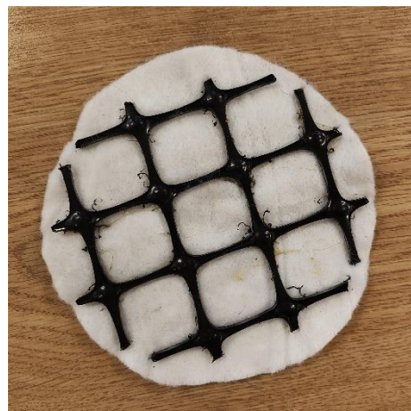
b) Wicking nonwoven geotextile-geogrid composite
