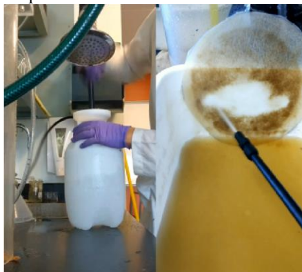
Fig.2. Washing method used for the non-woven geotextile.
