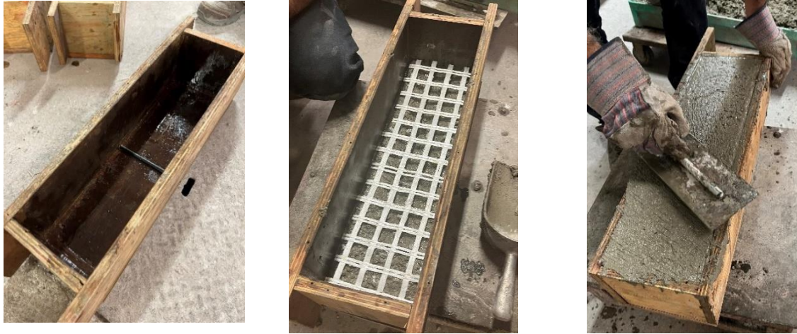
Fig. 2. Casting process for concrete specimens: a) prepare the wooden mould, b) place the geogrid layer, c) surface finishing.
