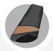
**3. SOLIDS REMAINS**As liquid escapes, the solids consolidate in the tube for eventual disposal.
