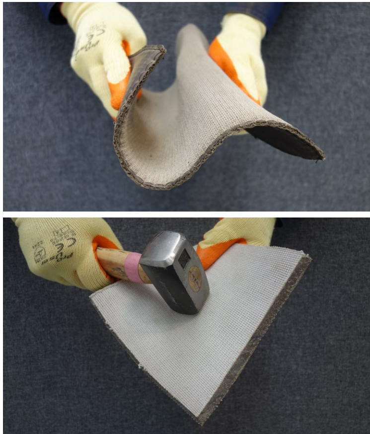
Figure 1. The change of GCCM properties from flexible to rigid on curing means that when assessing GCCM properties, appropriate test methods should be used to determine the cured, in-service GCCM cementitious layer performance.
