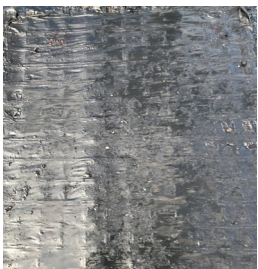
Close up of Titan’s new TE-FGP11-EPM geogrid showing desired melt of the bonding layer upon paving.
