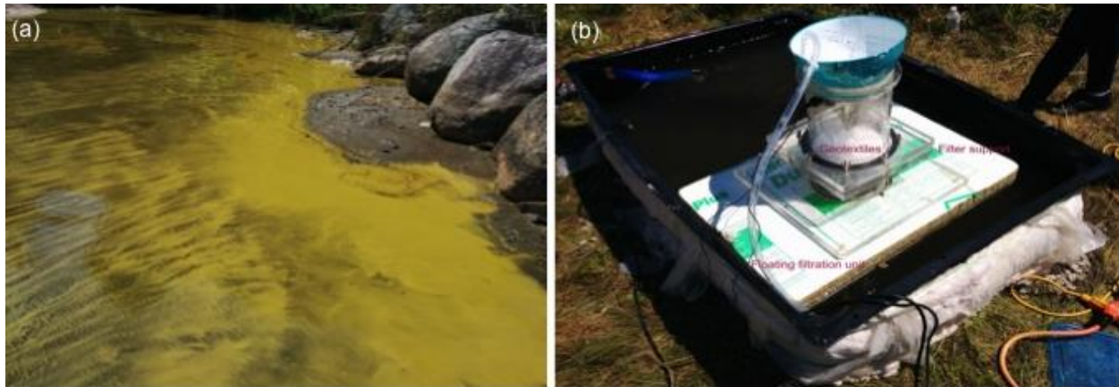
Figure. 1: (a) Algal bloom in Lake Caron (2016); (b) On-site floating geotextile filtration unit
