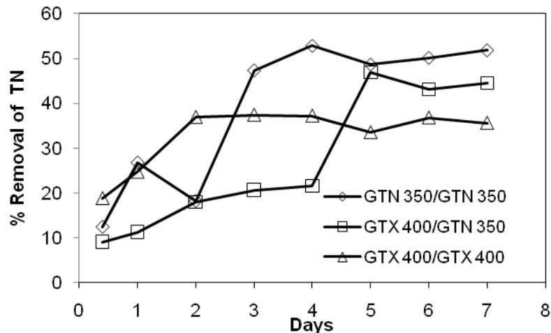
Figure 7. Efficiency of geotextile filters in removal of TN (%) over time
