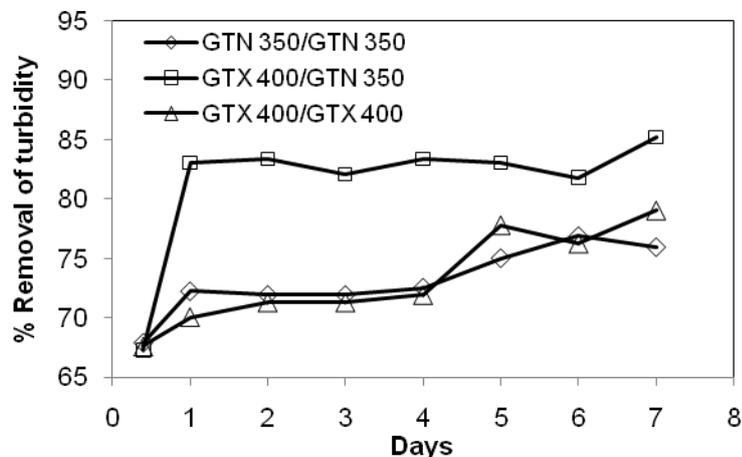
Figure 6. Removal of turbidity (%) over time by the geotextile filtration unit
