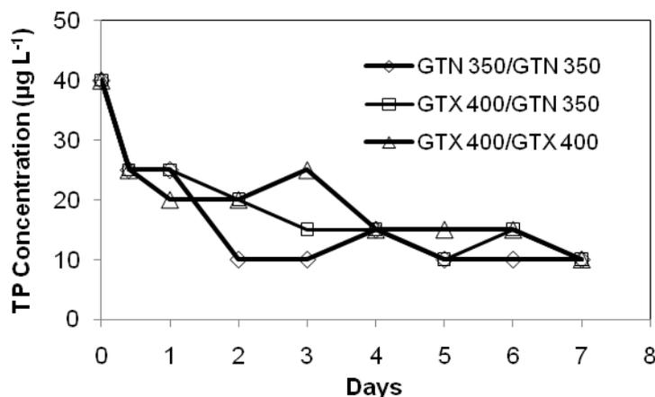
Figure 4. Changes in TP concentration ( $\mu\text{g L}^{-1}$ ) of lake water during the filtration by geotextile unit
