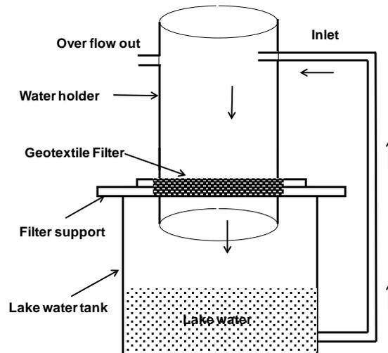
Figure 2. A schematic diagram of geotextile filter unit employed in the P removal from lake water
