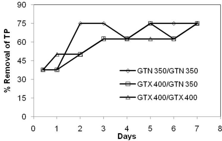
Figure 5. Removal of TP (%) over time by the geotextile filtration unit
