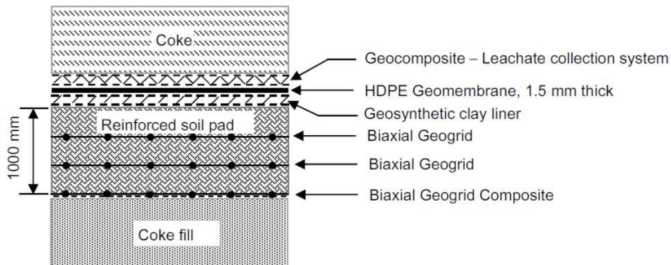
Figure 2. Components of the Lining system
