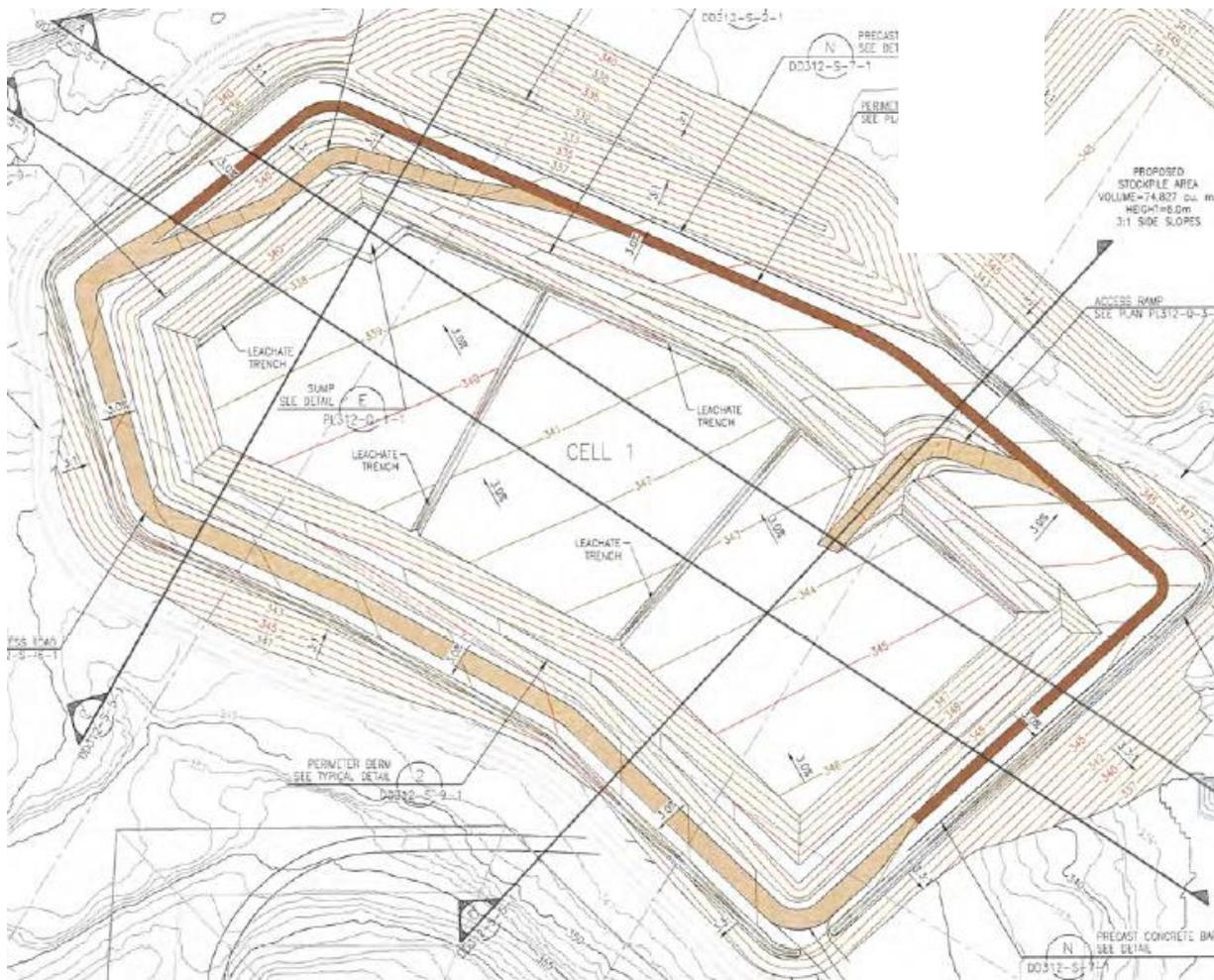
Figure 1. Plan and representative cross-sections of the coke landfill
