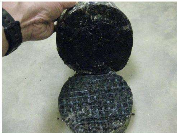
Figure 11 - Typical failure mode by slipping at the interface between fiberglass grid and nonwoven geotextile
