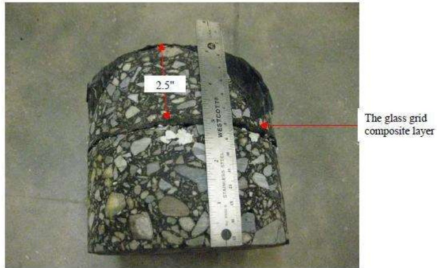
Figure 10 - Asphalt concrete core with fiberglass grid composite layer
