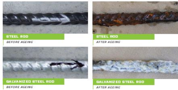
Figure 3. Steel Rod before and after aging test.
