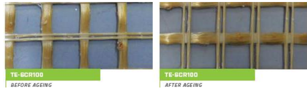
Figure 4. ConForce Grid before and after aging test.
