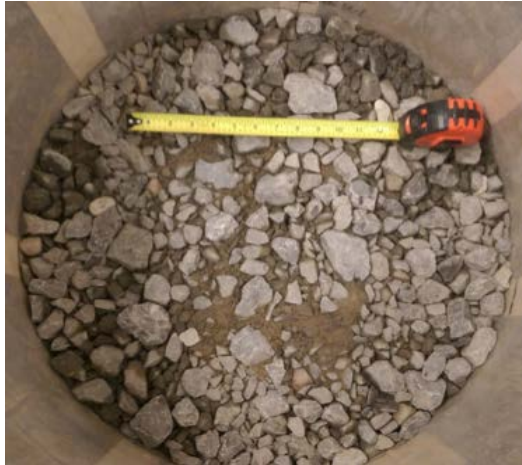
Figure 4. Underliner gravel used (overliner was essentially the same).
