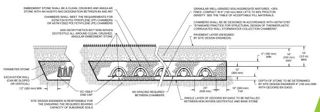
$^*MINIMUM\ COVER\ TO\ BOTTOM\ OF\ FLEXIBLE\ PAVEMENT.\ FOR\ UNPAVED\ INSTALLATIONS\ WHERE\ RUTTING\ FROM\ VEHICLES\ MAY\ OCCUR,\ INCREASE\ COVER\ TO\ 20"\ (510\ mm)$
