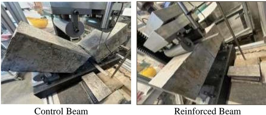
**Fig. 4.** Failure modes for control and reinforced beams
